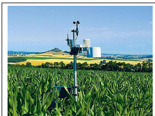
Station météo. Source: Next farming (France)
