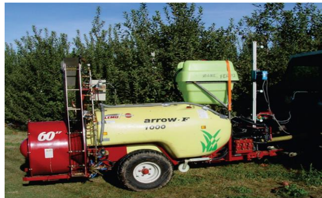
Ultrasonic and LIDAR sensors equipped air assistance sprayer. Source: Petrovic et al (2018)
