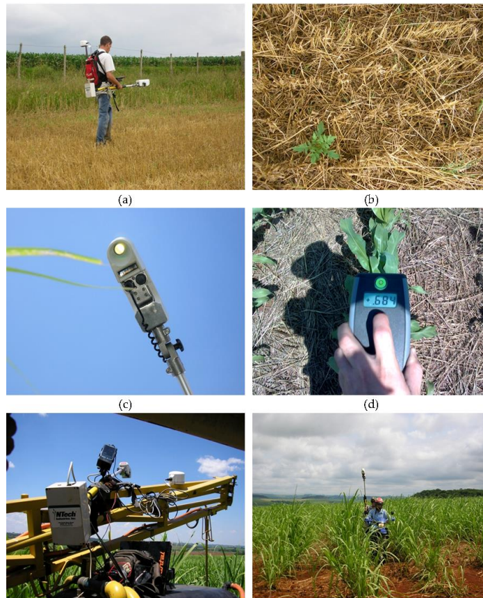
GreenSeeker sensor collecting NDVI values for weed (a) and (b); detailed pictures from GreenSeeker Hand Held (c) and Pocket Sensor (d); and GreenSeeker mounted on a sprayer (e) and on a motorcycle (f) collecting NDVI values in sugarcane.
