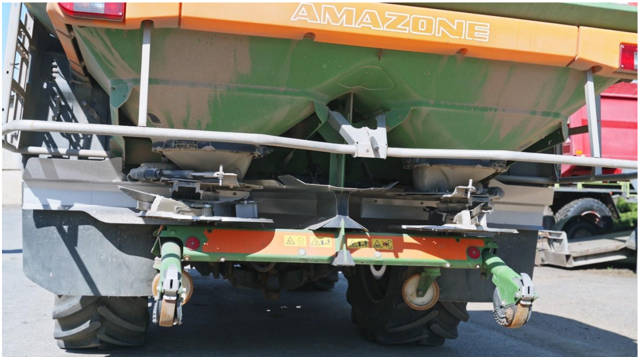
Figure 2 a, b : Smart adjustable machine blades for precise fertiliser application.
