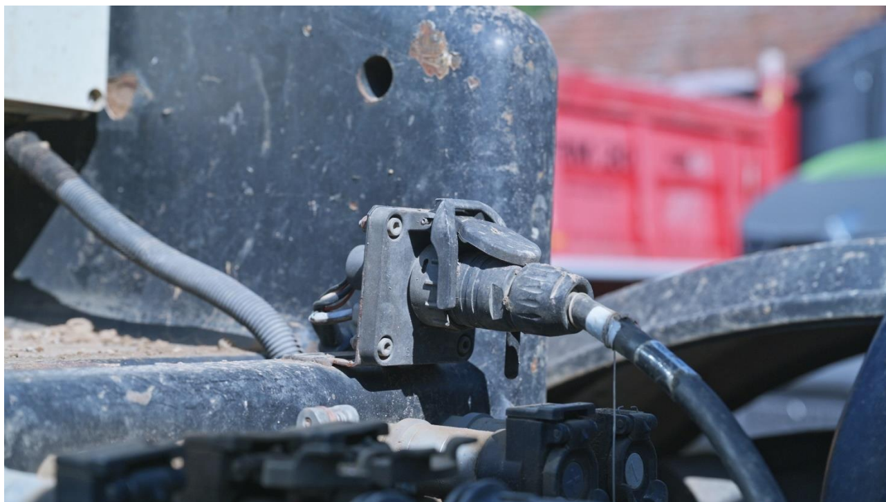
Picture 4 : ISOBUS connector to provide tractor and machine communication for precision fertiliser application.
