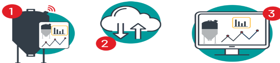
Figure 3: Steps in data collection by SiloSpi; silo, to sigfox cloud, to web/app
