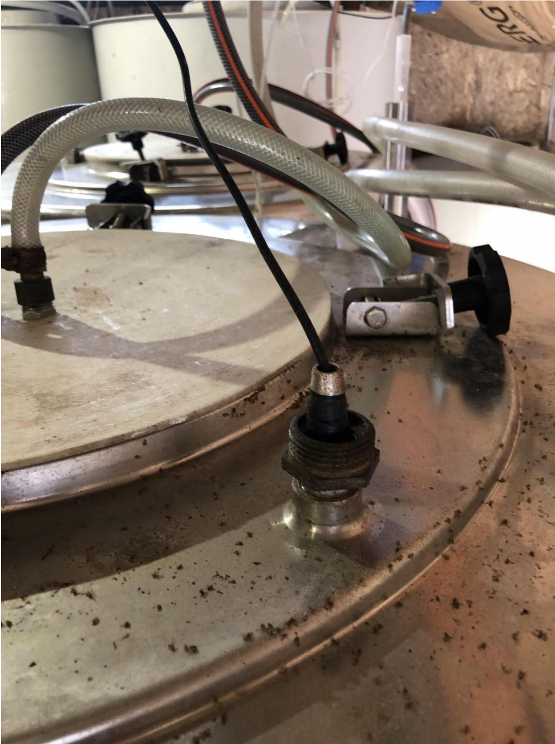
Temperature sensor installed to barrel
