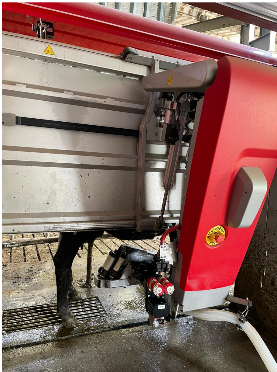
The red and white cylinders are used to clean the teat of the cow.
